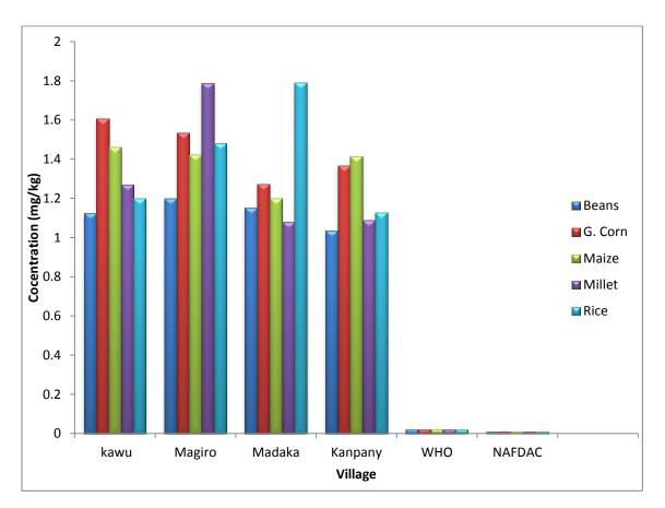
Figure 3. The concentration of Pb crop grains obtained from the communities around the mine site
